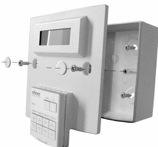
To open the housing, proceed as shown in the illustration. The plastic covers for the mounting bolts of the front panel will be pressed into the milling holes during final assembly. Therefore it is very difficult to remove them, and the covers will be damaged during disassembly. The housing therefore contains 3 additional replacement covers.
