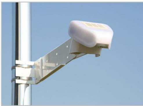
Ex. 2: Fitting to a pole with worm drive hose clips.
